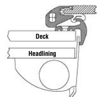
Cross Section of Roller Shade/Screen
